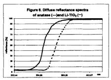
and anatase are shown in Figure 8. Li-TiO<sub>2</sub> shows a shift in the band edge, thus the band gap energy of this material which equals 3.9 eV is 0.7 eV higher than for anatase (3.2 eV).
