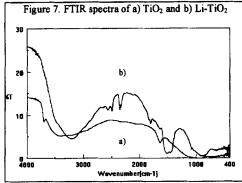
FTIR analysis also confirmed changes in the  $TiO_2$  structure (Figure 7). The new absorption bands appeared in the range of 2700 - 2250 cm<sup>-1</sup> and broad bands in the ranges of 1600 - 1300
