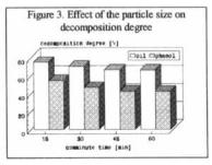
1.5 h and the catalyst content was 0.4 g dm<sup>-3</sup>. The complete oil decomposition was achieved after 2 h illumination, while the complete decomposition of phenol in water was achieved after 2.5h of illumination with the same catalyst content. Decomposition degrees of phenol and oil (the same reaction conditions) using pure titanium dioxide were 42% and 68%, respectively.
